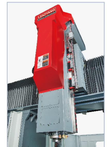
Available to mount with linear guideways on Z-axis and use direct-drive high speed spindle (8,000~15,000 rpm) (optional).
