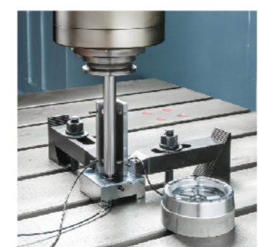
Thermal growth compensation device for spindle
